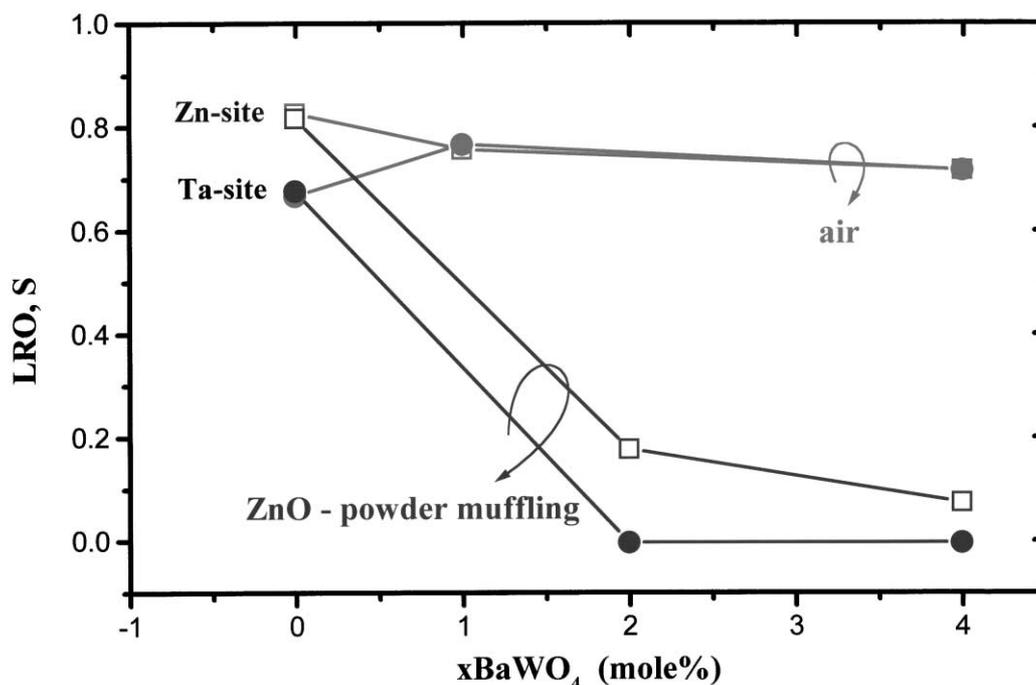
Fig. 5. Effect of sintering atmosphere and  $\text{BaWO}_4$  dopant on LRO parameter ( $S$ ).  $S$  was calculated from the refined occupancies of the Zn and Ta-sites. [ $S = (R_A - F_A) / (1 - F_A)$ ;  $R_A$ , A atom on the ordered position;  $F_A$ , fraction of A atoms].
