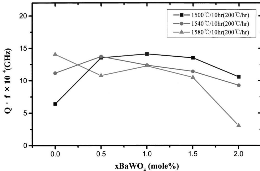
Fig. 3. Effect of sintering temperature and  $\text{BaWO}_4$  doping on the  $Q \cdot f$  values. The specimens were sintered for 10 h at each temperatures; the heating rate was 200 °C/h.
