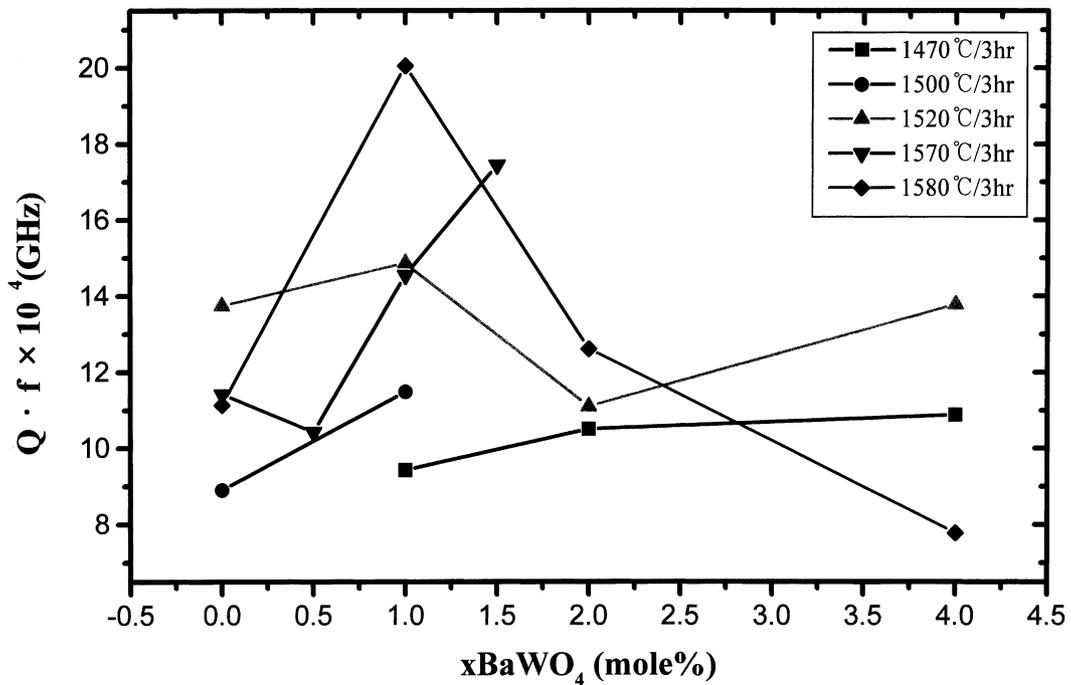
Fig. 2. Variation of  $Q \cdot f$  values with sintering temperature and the  $\text{BaWO}_4$  content. The specimens were sintered for 3 h at each temperatures.
