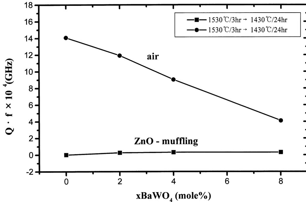
Fig. 1. Effect of sintering atmosphere on the  $Q \cdot f$  values. Samples were sintered at 1530 °C for 3 h and post-annealed at 1430 °C for 24 h either in air or ZnO-powder muffling.
