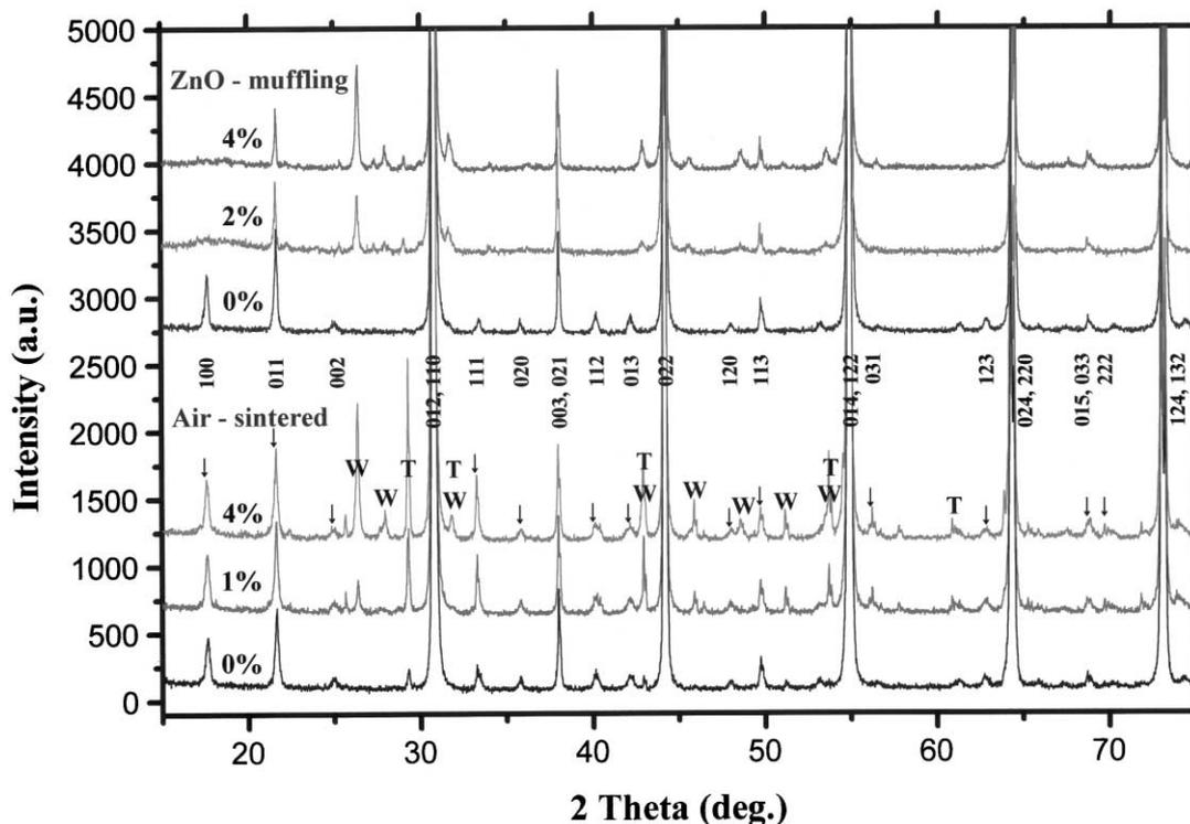
Fig. 6. X-ray diffraction patterns of the  $\text{BZT}-(0, 1, 2, 4)$  mol%  $\text{BaWO}_4$  sintered in either air or in ZnO-powder muffling at  $1530^\circ\text{C}$  for 3 h and post annealed at  $1430^\circ\text{C}$  for 24 h. (T,  $\text{Ba}_7\text{Ta}_6\text{O}_{22}$ ; W,  $\text{BaWO}_4$ ).
