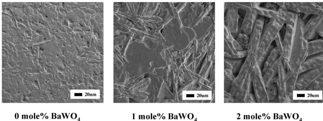
Fig. 4. SEM micrographs of the BZT-(0, 1, 2) mol%  $\text{BaWO}_4$  sintered in air for 10 h at 1540 °C.
